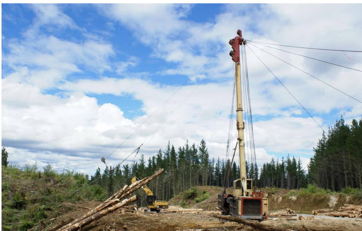
Pictured: A swing yarder in operation
