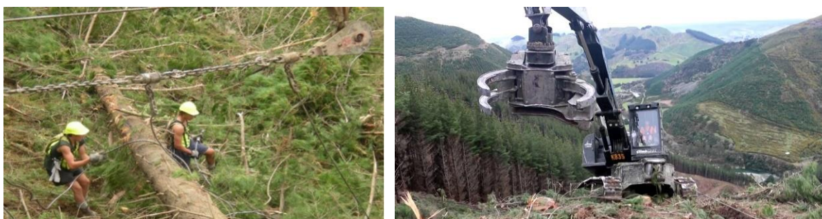
Pictured: forestry workers breaking out with winch, line hauler, and harvester head
